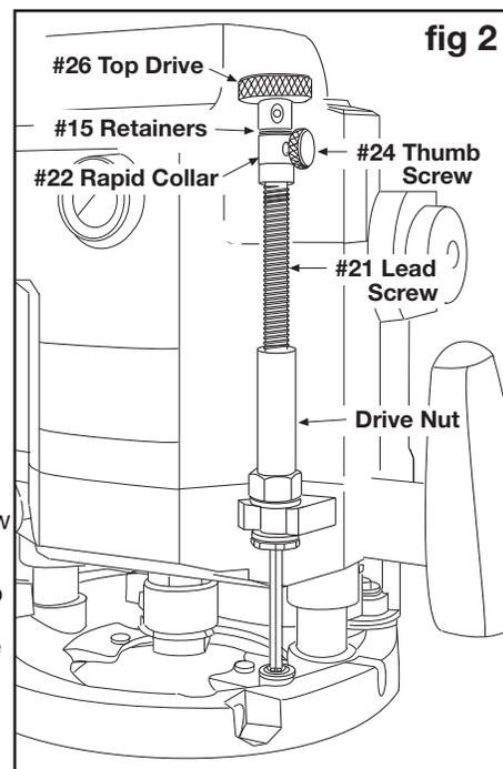
**Caution:** #22 rapid collar is not designed to maintain cutter height during routing operations. Always secure plunge lock before and during all routing operations.
