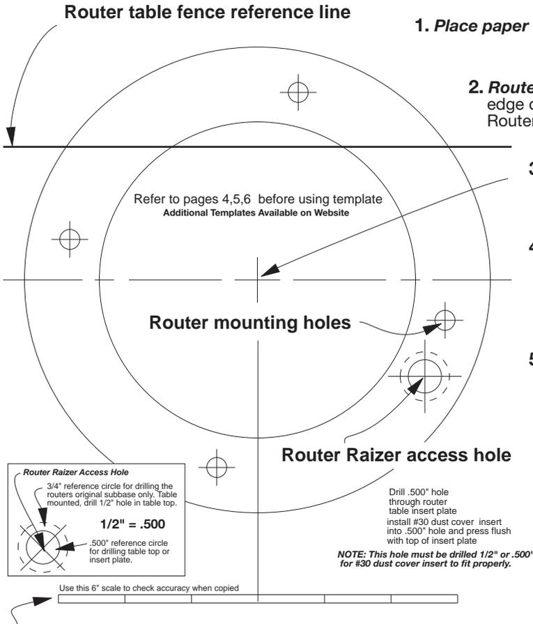
1. Place paper template lettering up onto top side of router table or inset plate.
