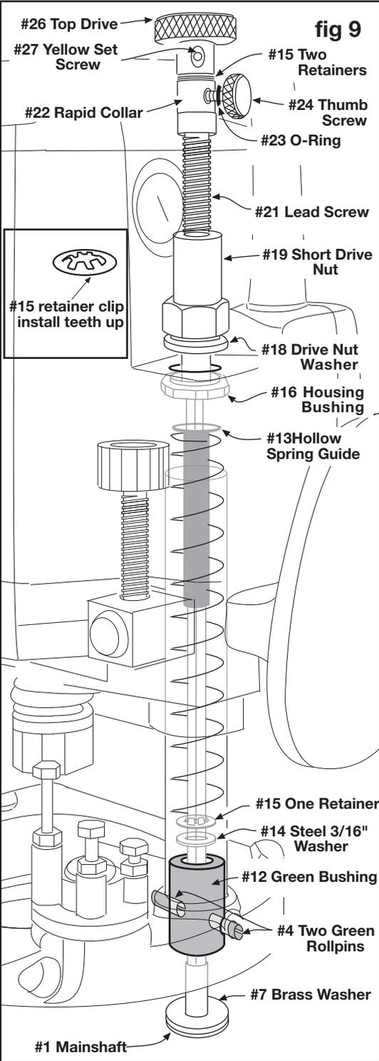
3. Select #11 blue bushing, ( Two #15 retainers ) #21 lead screw, #22 rapid collar, #23 O-ring, #24 thumb screw, #25 black set screw, #26 top drive, #27 yellow set screw, #28 allen wrench, red grease. Using ( fig 9 ) place grease on threads of #21 lead-screw, Place lead screw down #1 mainshaft and thread into #19 short nut until one inch of mainshaft extends above head of #21 lead screw. **Alignment of #1 mainshaft and #21 screw hex is required ( fig 10 ).**
