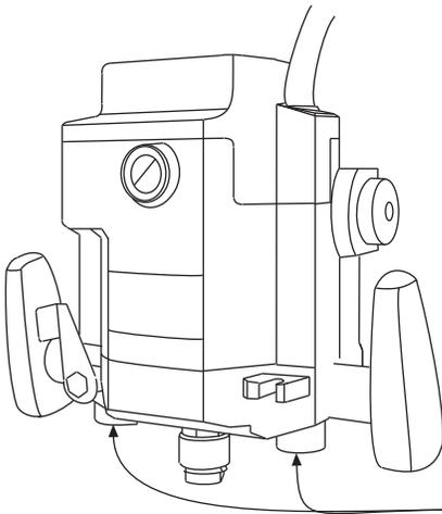
Post Bushings Apply light film on the inside surface of both post bushings.
