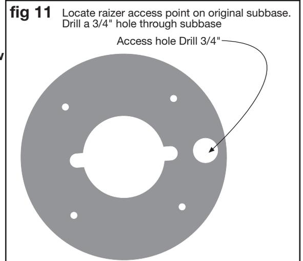
**NOTE: This router requires a 3/4" pocket or use of 8" X 8" black rubber spacer for router table installation. Pages 4,5,6.**
