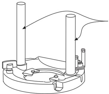
Plunge Posts Apply light film to the outside surface of both plunge posts.
