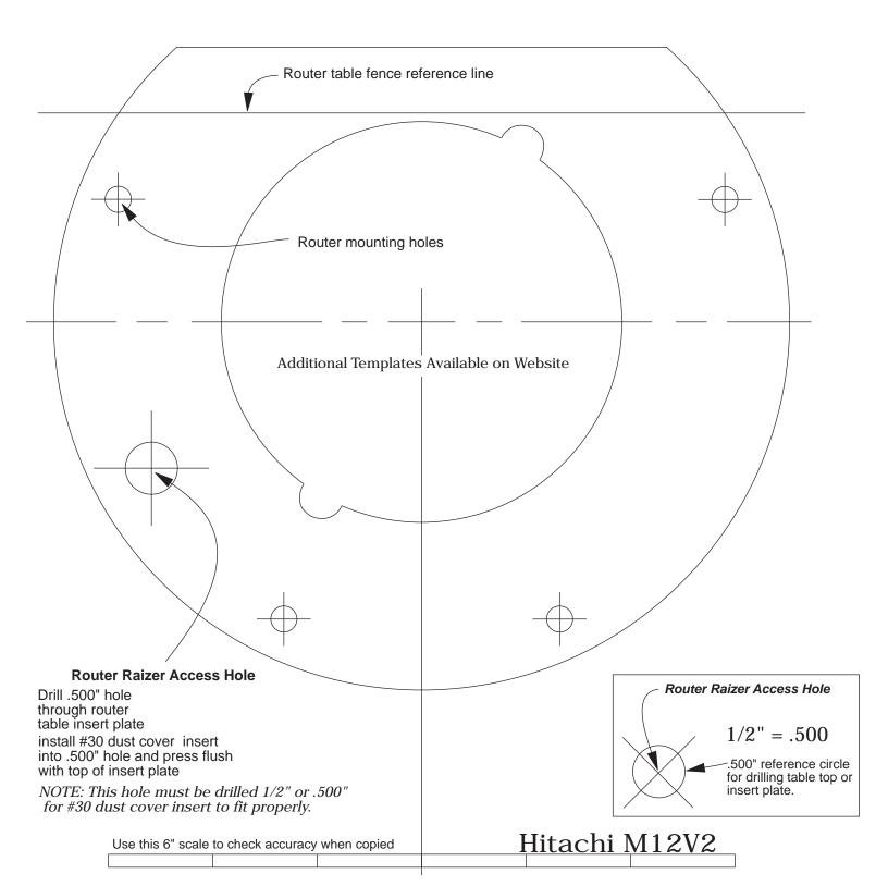
**Note:** Cross lines for locating and drilling holes are accurate. The illustration of subbase may vary slightly in size and design, but is accurate enough for cutting the rubber spacer if required.
