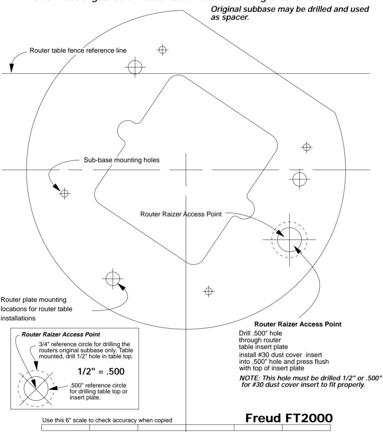
**Note:** Cross lines for locating and drilling holes are accurate. The illustration of subbase may vary slightly in size and design, but is accurate enough for cutting the rubber gasket if required.
