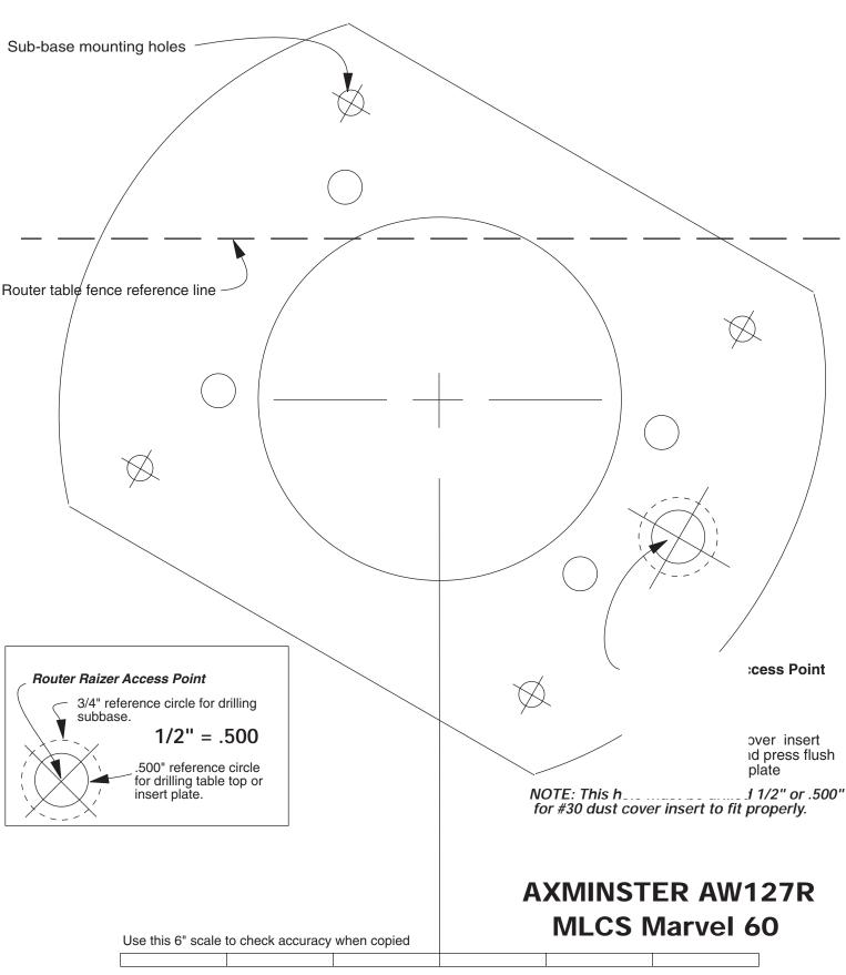
*Note:* Cross lines for locating and drilling holes are accurate. The illustration of subbase may vary slightly in size and design, but is accurate enough for cutting the rubber gasket if required.
